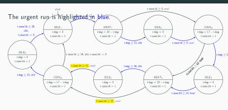
When the HA is in  $COOL_4$ , it's 2 hours to midnight and we need slightly less of that amount of time to lower the temperature from  $24^{\circ}$  to  $18^{\circ}$ .
