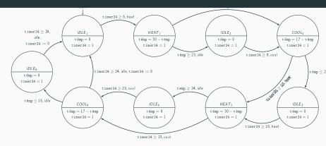
Considering urgency of transitions, does there exist a situation in which the HA cannot reach the desired temperature in time?
