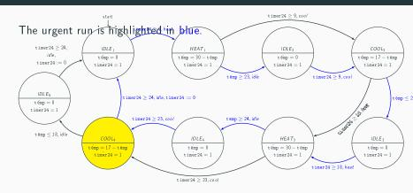
When the HA is in  $COOL_4$ , 1 hour is a time too short to lower the temperature from 23° to 18°.
