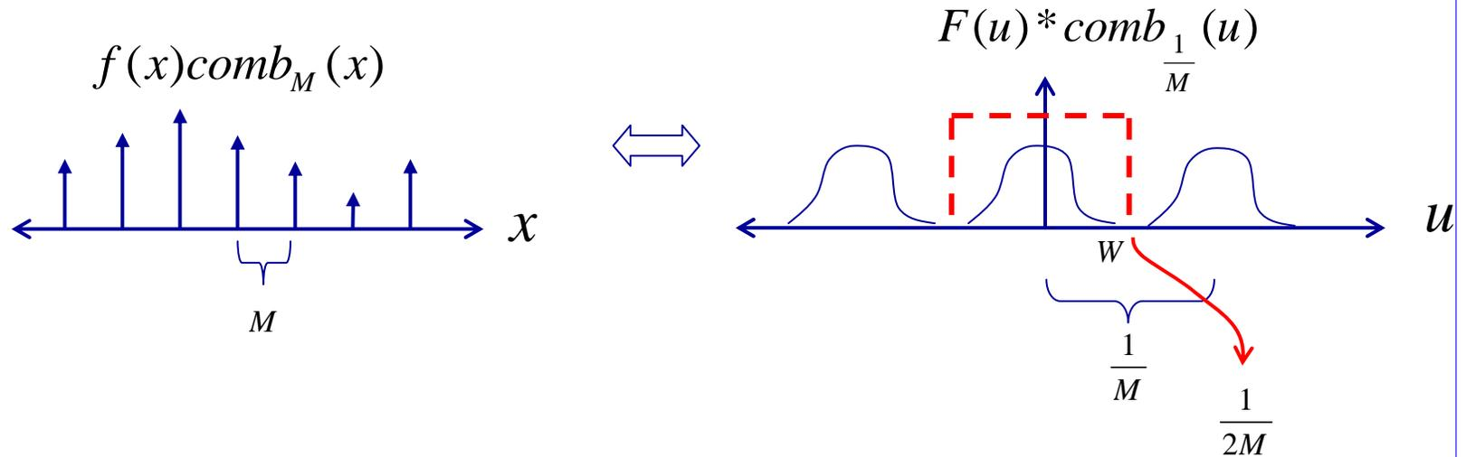
*If there is no aliasing, the original signal can be recovered from its samples by low-pass filtering.*
