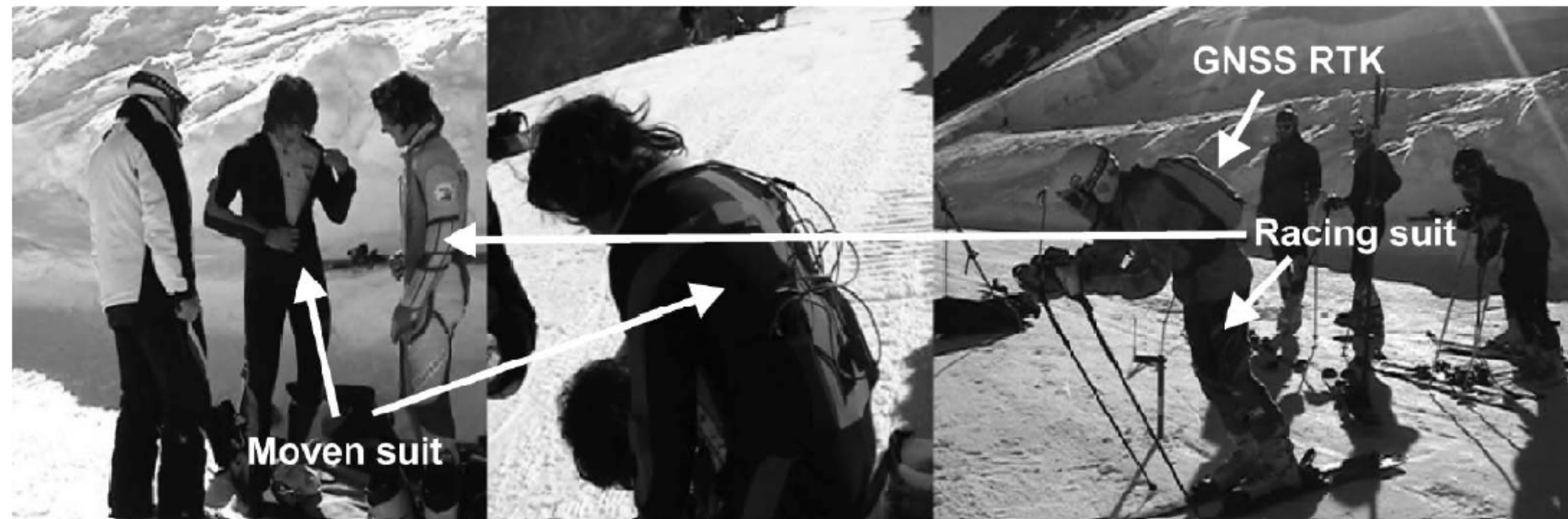
Figure 2. The Moven suit consisted of 16 inertial motion-tracking sensors, embedded in a lycra suit worn under the skier's skin-tight ski racing suit. The RTK GNSS receiver, data logger, and antenna are housed in a small backpack worn by the skier.
