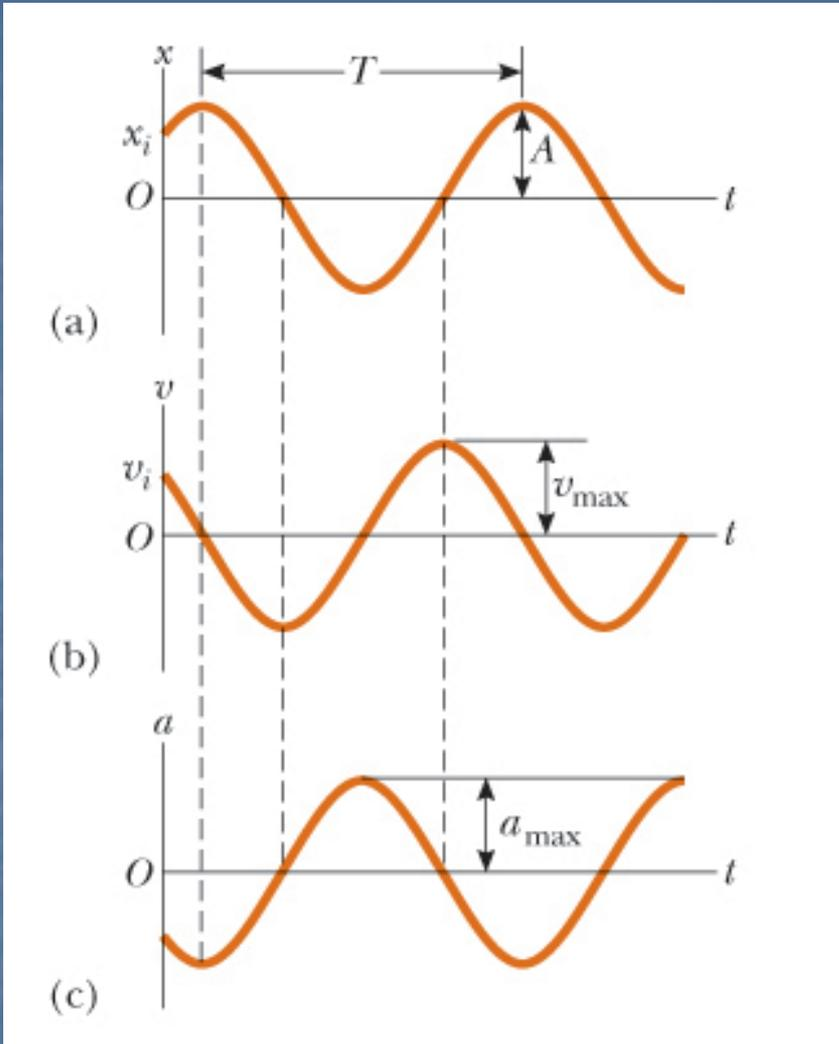
$$v = \frac{dx}{dt} = -\omega A \sin(\omega t + \phi)$$
