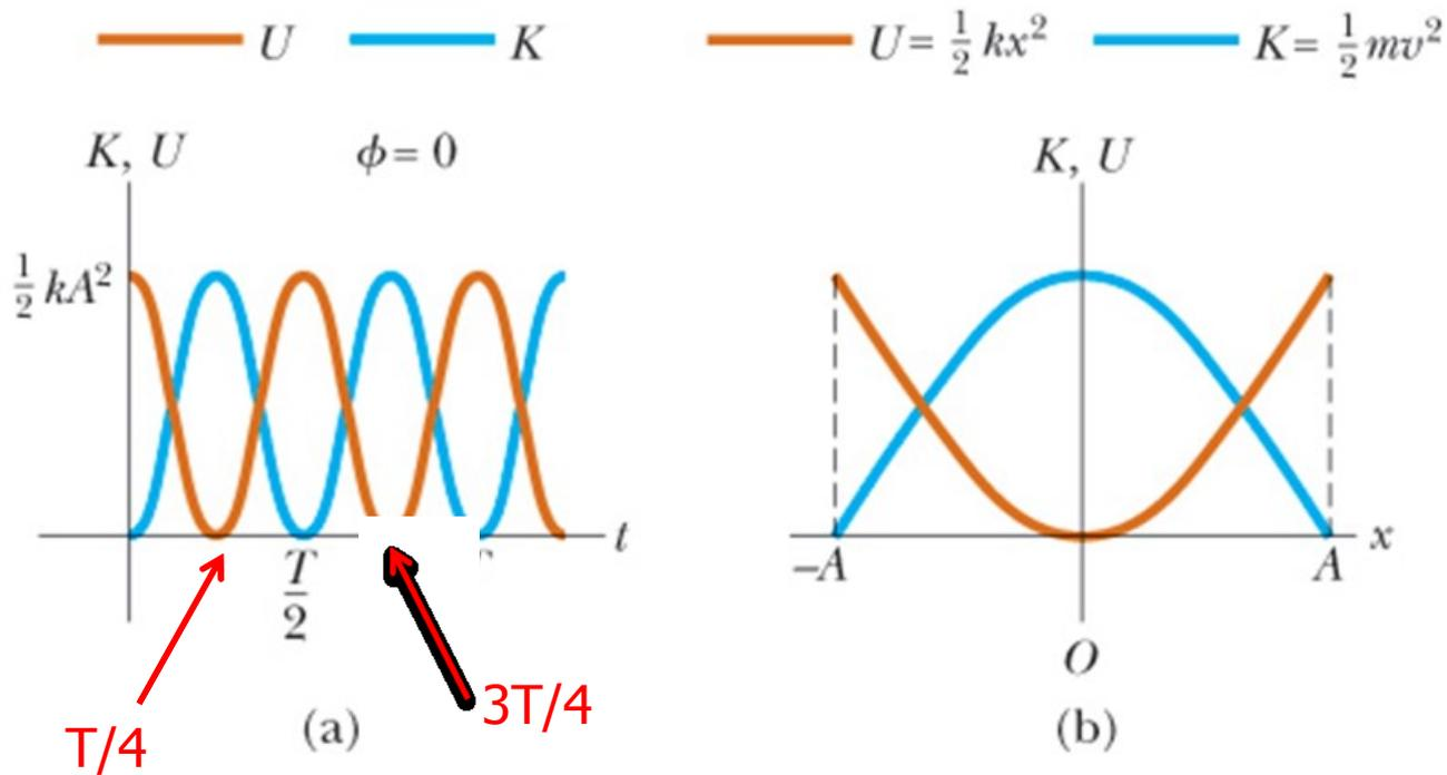
$$E = K + U = \frac{1}{2} k A^2 \sin^2(\omega t + \phi) + \frac{1}{2} k A^2 \cos^2(\omega t + \phi)$$
