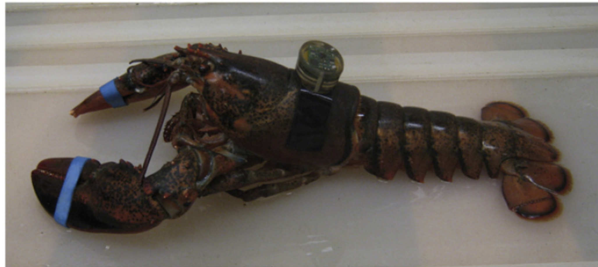
Fig. 1. Tri-axial accelerometer data logger attached directly to the dorsal carapace surface of a lobster using industrial strength Velcro® and adhesive.
