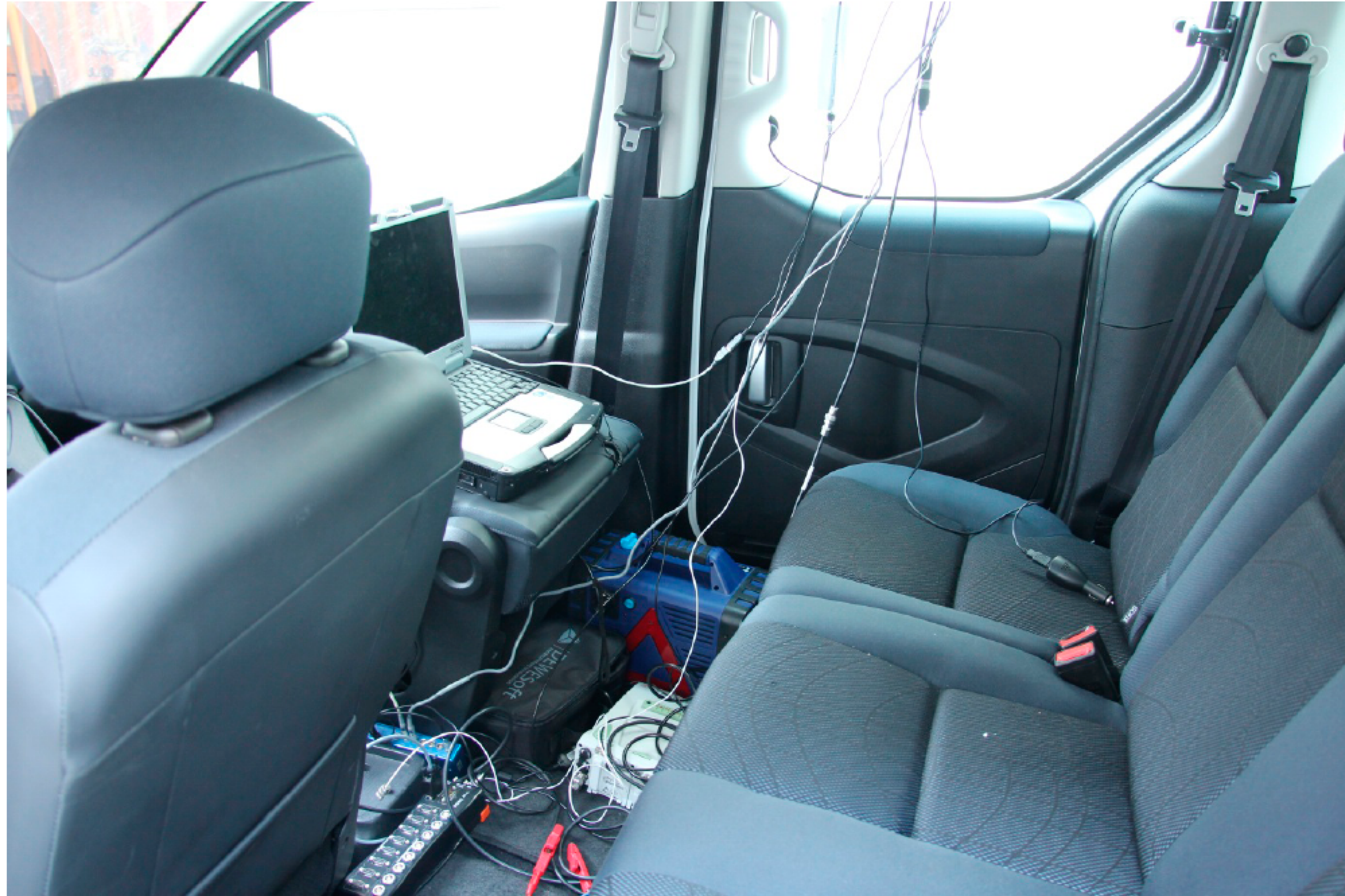
Figure 2. Laptop with the external analog-digital unit in the vehicle synchronously stored data from two GNSS systems and the vehicle speedometer.
