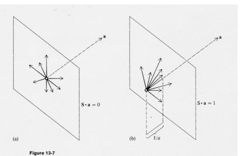
The von Laue scattering conditions for a one-dimensional array. Scattering vectors are shown as solid arrows. (a) For  $\mathbf{S} \cdot \mathbf{a} = 0$ . (b) For  $\mathbf{S} \cdot \mathbf{a} = 1$ .
