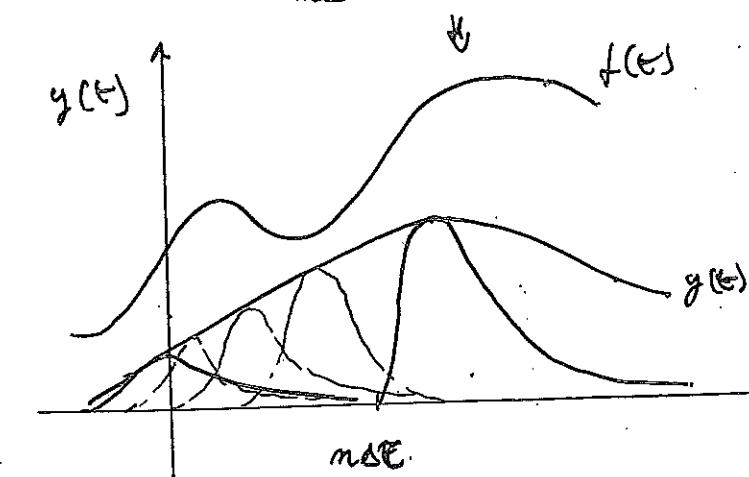
$y(t)$  is obtained by summing the responses to the impulses  $\rightarrow$  The envelop of the corresponding set of curves.
