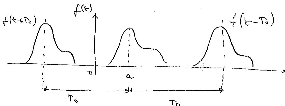
$T_0 \rightarrow \infty$  The spacing sums up the pulses increases and in the limit  $T_0 \rightarrow \infty$ , we find the original function
