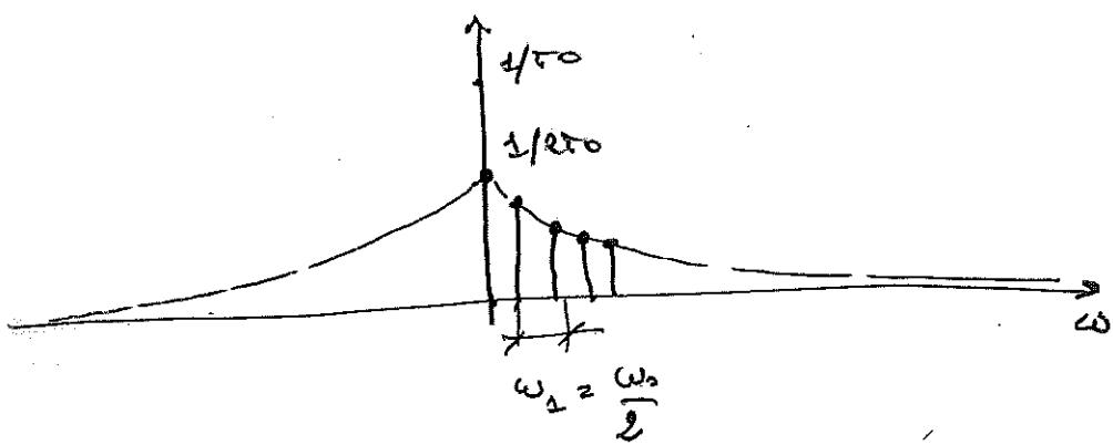
⇒ When  $T_0 \uparrow$ ,  $\omega_0 \downarrow \Rightarrow$  The sampling of the spectrum becomes denser and the amplitude decreases.
