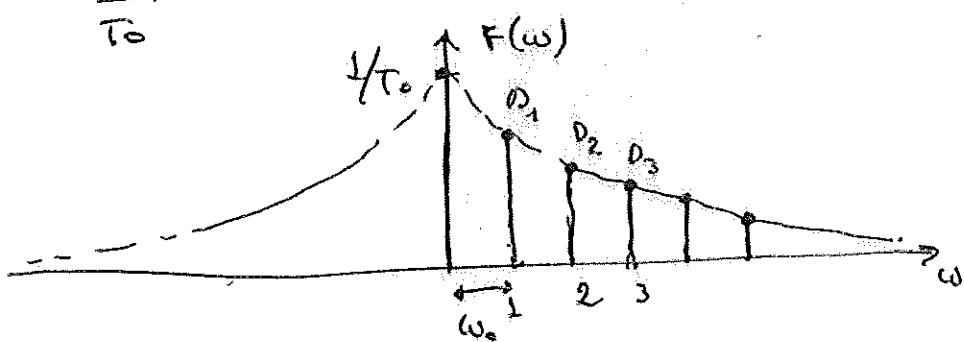
$$T_1 = 2T_0 \rightarrow \omega_1 = \frac{\omega_0}{2} \rightarrow D_m^1 = \frac{1}{T_1} F(m\omega_1) = \frac{1}{2T_0} F(m\omega_0)$$
