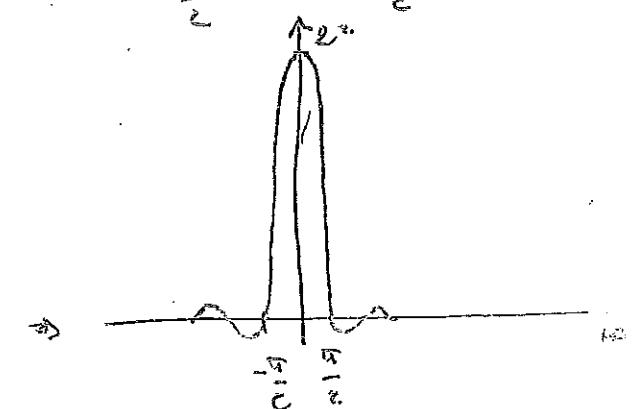
$$\alpha = \frac{c}{2} \Rightarrow F_B(\omega) = 2 F_L(\omega) = 2 \sin(\omega c)$$
